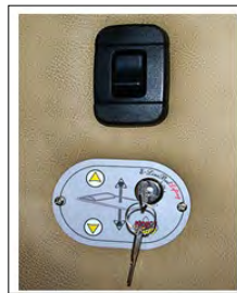
Fig 3: Key ON (Horizontal)
